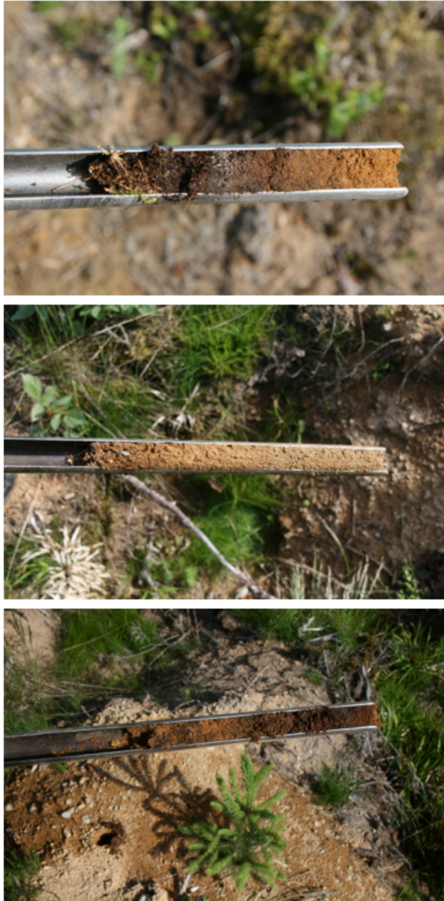
Figure 2 The different soil surface disturbance classes; undisturbed (top), pit (center) and mound (bottom). The soil surface layer structure in the undisturbed soil consist of an intact organic layer and mineral soil layers. The soil cores illustrate that the dark organic layer is missing entirely from the pits and in the mound, organic matter has been mixed with the mineral soil. (Photos: Heljä-Sisko Helmisaari and Mikael Marjanen)
