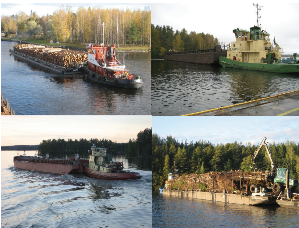
Figure 18. Alternative tugboat and barge combinations in Finland (the systems on the right side were used in the demonstration and simulation) (K.Karttunen).
