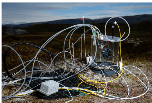
Figure 2: Chamber setup during measurement period, with soil moisture and soil temperature sensors installed in the soil, and all inlets connected. Photo: Fabio Cian, "Ubiquitous Anomaly", CC BY-NC-ND 4.0 ( I )
