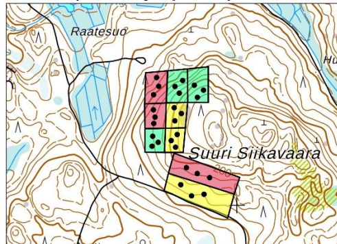
Figure 4. Set-up of the N-fertilization experiment with three target N-doses (0, 150 and 200 kg N ha -1 ) in four research sites. Each site contained nine blocks, to which the target N-dose was randomly selected. The green color indicates control blocks, yellow indicates treatment of 150 kg N ha -1 , and red 200 kg N ha -1 . Three plots were randomly located inside each block. The base maps are retrieved from open data of the National land survey of Finland ( https://asiointi.maanmittauslaitos.fi/karttapaikka/?lang=en ).
