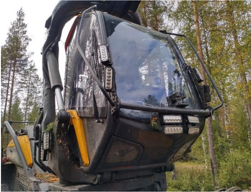
Figure 2. The cabin of a Ponsse Scorpion King harvester. The Ouster LiDAR OS0 is mounted on a bar located beneath the front windshield. Photo courtesy of Johannes Pohjala
