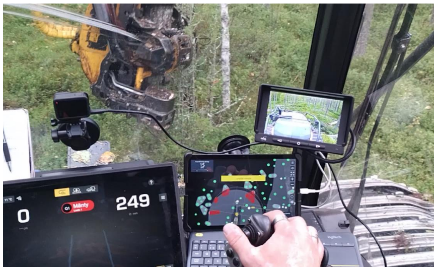
Figure 3. An operator's view showing the Opti-5G system of a Ponsse machine, with a GoPro Hero 8 camera mounted on the windscreen with a suction cup. A Ponsse Thinning Density Assistant (TDA) display is positioned in the centre, and a reversing camera is positioned on the pillar. Photo courtesy of Johannes Pohjala
