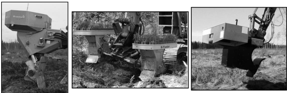
Figure 2. Planting devices in use today: Bracke P11.a (left, photo: Mikko Syri), M-Planter (middle, photo: Heidi Hallongren), and Risutec TK-200 (right, photo: Jussi Aikala)
